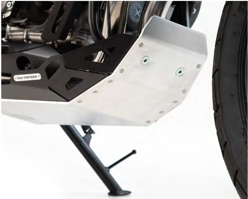
Above: Discreet engine guard for the BMW R nineT Right: Engine guard in two different colors - brushed aluminum and powder coated black
