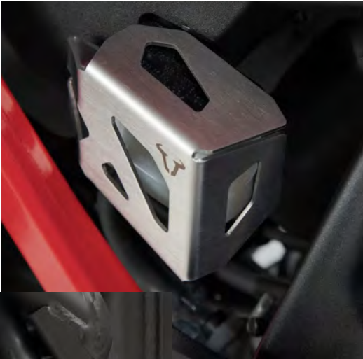
Water pump protection on the Ténéré 700 (left) and brake reservoir guard on the Africa Twin CRF 1100 (below)
