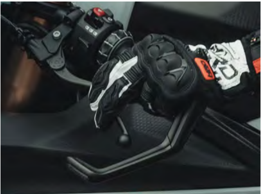
Protection for brake lever and clutch lever
