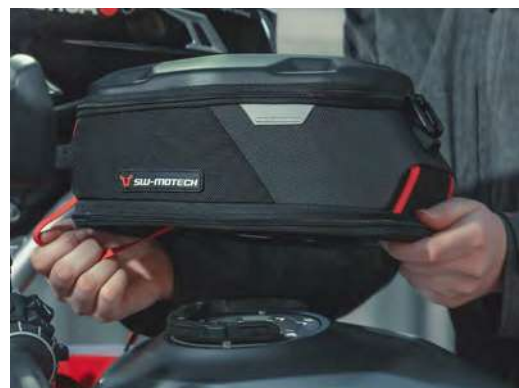
Easy attachment thanks to the magnetic guide
