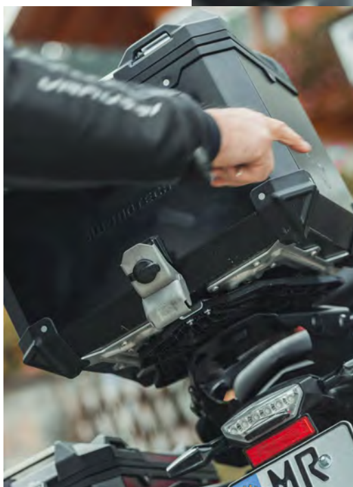
A lock in the latch buckle secures the top case against theft
