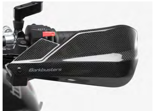
Handguard shells made from carbon fiber
