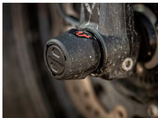
Fiberglass-enforced plastic with TPE sheathing for high mechanical dampening capacity
