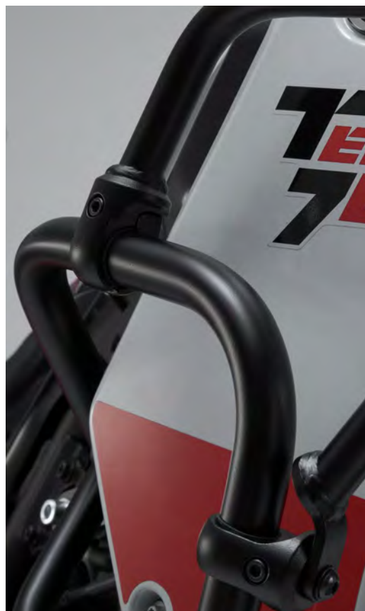
Fitted crash bar clamps for a secure hold.
