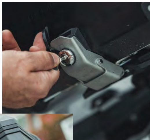
A lock in the latch buckle secures the top case against theft
