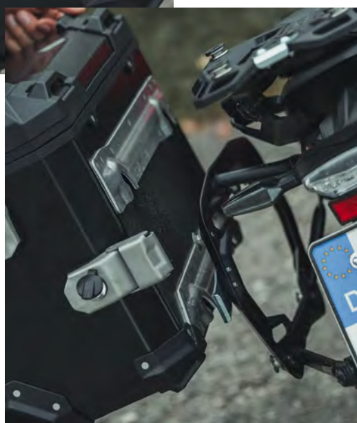
The side cases clip securely and easily into the four retention spoons mounted on the carrier.
